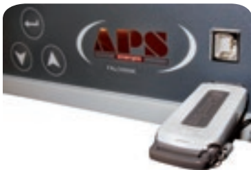
The USB type port (B) sends archive data directly to a PC
