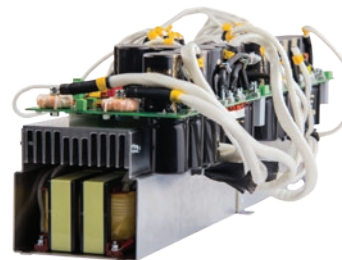
View of the PBI rectifier power block
