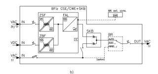
Fig. 71. Block diagram of the BFIz type inverter compact with a power supply unit and the SKB type bypass: a) with a built-in console; b) with an external MK console.
