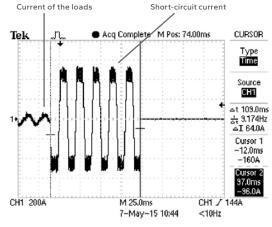
Oscillogram of the programmed current and the duration of short-circuit of the inverter
