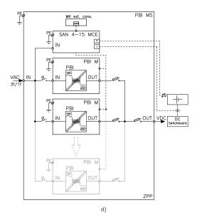
Fig. 14. Block diagram of the PBI type rectifier cabinet (on the basis of the PBI M modules) for parallel operation:
