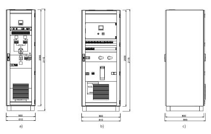
Fig. 84. Views with dimensions of the static switch cabinet:
