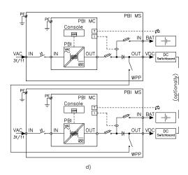
Fig. 13. Block diagram of the PBI type rectifier cabinet (on the basis of the PBI MC modules) for parallel operation: a) the PBI MC system with WPP for operation with a single battery; b) the PBI MC system with WPP for operation with two batteries; c) the PBI MC system with ZPP; d) the PBI MS system for operation with two batteries.
