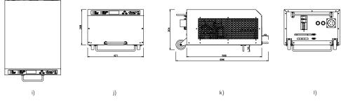
Fig. 19. Views with the dimensions of the PBI type rectifier compact (wall-mounted and portable enclosure): a) CW4 compact – front view; b) CW4 compact – left-side view; c) CW6 compact – front view; d) CW6 compact – left-side view; e) CW7 compact – front view; f) CW7 compact – left-side view; g) CW8 compact – front view; h) CW8 compact – left-side view; i) CP compact – top view; j) CP compact – front view; k) CP compact – left-side view; l) CP compact – back view.
