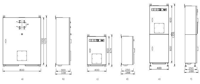
Fig. 86. View with dimensions of the SKB type static switch compact: a) CW1 compact – front view; b) CW1 compact – left-side view; c) CW4 compact – front view;
