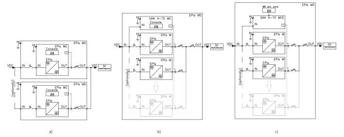
Fig. 36. Block diagram of the EPIs type converter cabinet for parallel operation: a) a system with EPIs MC; b) a system with EPIs M and an external SAN 4-15 MC controller with a built-in console; c) a system with EPIs M and an external SAN 4-15 MCE controller with an external MK console.
