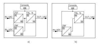
Fig. 100. General block diagram of the asynchronous motor power supply system: a) with the FATz type power supply unit; b) without the FAT type power supply unit.
