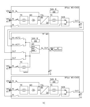
Fig.68.BlockdiagramoftheBFlpztypeinvertercabinetsinafreedesignforparalleloperation with the SKB type bypass and the TP type distribution board. Possible configurations: a) a parallel system of two BFlpz inverters with own SKB and maintenance bypasses – two AC reserve power supplies in the TP cabinet;
