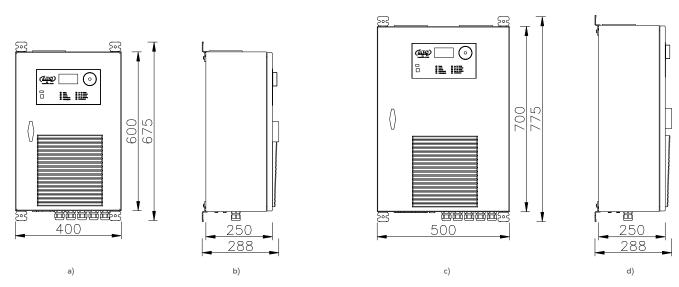
Fig. 41. Views with dimensions of the EPI type converter compact (wall-mounted enclosure): a) CW4 compact – front view; b) CW4 compact – left-side view; c) CW6 – front view; d) CW6 compact – left-side view.
