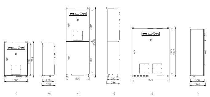
Fig. 73. Views with dimensions of the BFIz / BFI type inverter compact: a) CW6 compact – front view; b) CW6 compact – left-side view; c) CS6 compact – front view; d) CS6 compact – left-side view; e) CW1 compact – front view; f) CW1 compact – left-side view.
