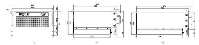
Fig. 57. Views with dimensions of the BFlpz / BFlp M type inverter module:
