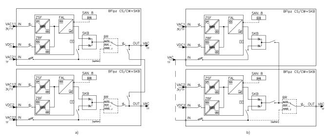
Fig. 74. Block diagram of the BFlpz inverter compact for parallel operation with a power supply unit and the SKB type bypass. Possible configurations: a) two autonomous maintenance bypass switches, a built-in console; b) a common maintenance bypass switch, a built-in console.
