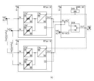
Fig. 49. Block diagram of the inverter module for parallel operation with the BFlpz power supply unit. Possible configurations: a) two autonomous SKB type bypasses, a console built in the inverter module; b) a common SKB type bypass, a console built in the MWB module.
