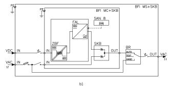
Fig. 60 a) and b) present a standard solution for single-phase module inverters in an industrial cabinet.
