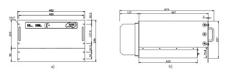
Fig. 11. Views with dimensions of the MP PBI type rectifier module in the M3-MP enclosure: a) front view; b) left-side view.
