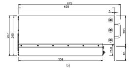
Fig. 103. Views with dimensions of the FATz / FAT MC type drive inverter: a) front view in the M5 enclosure; b) left-side view in the M5 enclosure.
