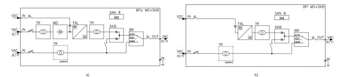
Fig. 61. Block diagram of the inverter cabinet in a free design: a) the BFIz type with the SKB bypass; b) the BFI type with the SKB bypass. Fig. 61 a) and b) present a standard solution for single-phase or three-phase inverters in a free design in an industrial cabinet.
