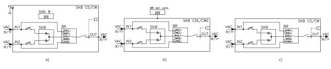
Fig. 85. Block diagram of the SKB type static switch compact: a) with a built-in console; b) with an external MK console; c) without a console.
