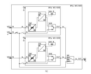
Fig. 63. Block diagram of the inverter cabinet consisting of the BFlpz/BFlp type inverter modules for parallel operation of max. module power up to 10kVA with the SKB type bypass (1-phase solution). Possible configurations:
