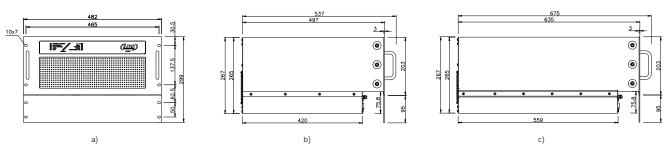
Fig. 94. Views with dimensions of the HPI type frequency converter module:
