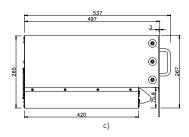
Fig. 10. Views with dimensions of the M/MC/MCE PBI rectifier module in the M3 enclosure: a) front view – a module with a built-in console; b) front view – a module without a console; c) left-side view.
