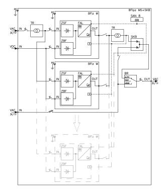
Fig. 66. Block diagram of the inverter cabinet consisting of the BFlpz type inverter modules for parallel operation of max. module power up to 15kVA with the SKB type bypass. A system with "n" module inverters with a common bypass (1-phase or 3-phase solutions).
