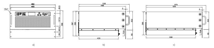
Fig. 51. Views with dimensions of the BFIpz / BFIp MC type inverter module (option): a) front view in the M3 and M5 enclosure; b) left-side view in the M3 enclosure; c) left-side view in the M5 enclosure.
