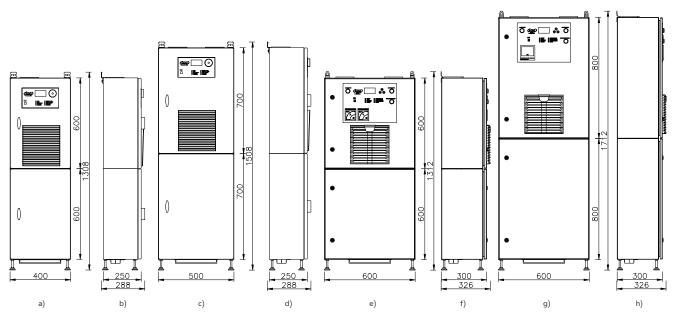
Fig. 18. Views with the dimensions of the PBI type rectifier compact (standing enclosure): a) CS4 compact – front view; b) CS4 compact – left-side view; c) CS6 compact – front view; d) CS6 compact – front view; e) CS7 compact – front view; f) CS7 compact – left-side view; g) CS8 compact – front view; h) CS8 compact – left-side view.
