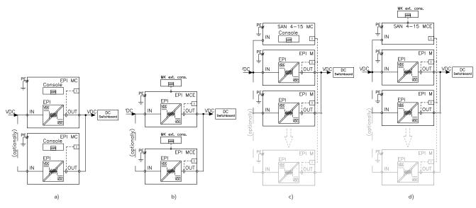
a) the EPI MC type modules system; b) the EPI MCE type modules system with an external MK console;
