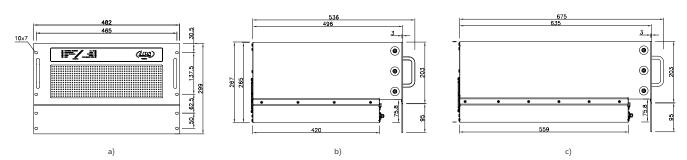
Fig. 59. Views with dimensions of the BFIz / BFI M type inverter module: a) front view in the M3 and M5 enclosure; b) left-side view in the M3 enclosure; c) left-side view in the M5 enclosure.
