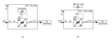
Fig. 38. Block diagram of the EPI type converter compact for autonomous operation: a) with a built-in console; b) with an external MK console.
