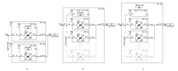
Fig. 35. Block diagram of the EPI type converter cabinet for parallel operation: a) a system with EPI MC; b) a system with EPI M and an external SAN 4-15 MC controller with a built-in console; c) a system with EPI M and an external SAN 4-15 MCE controller with an external MK console.
