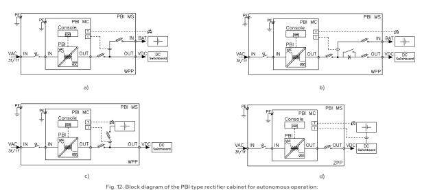
a) a system with WPP; b) a system with WPP and a counter cell; c) a system with WPP and an external battery in the rectifier's cabinet; d) a system with ZPP.
