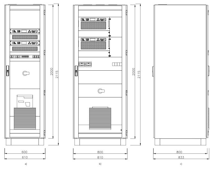
Fig. 37. Views with dimensions of the EPI / EPIs converter cabinet:
