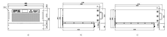
Fig. 58. Views with dimensions of the BFIz / BFI MC HC type inverter module: a) front view in the M3 and M5 enclosure; b) left-side view in the M3 enclosure; c) left-side view in the M5 enclosure.
