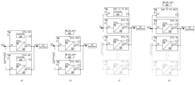
Fig. 30. Block diagram of the converter modules without the EPIs type insulation for parallel operation:
