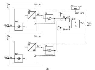
Fig. 56. Block diagram of the BFlp type inverter modules for parallel operation and the MWB module. Possible configurations: a) battery power supply, built-in console; b) battery power supply, external MK console;
