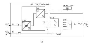
Fig. 72. Block diagram of the BFI type inverter compact with the SKB bypass: a) with a built-in console; b) with an external MK console.
