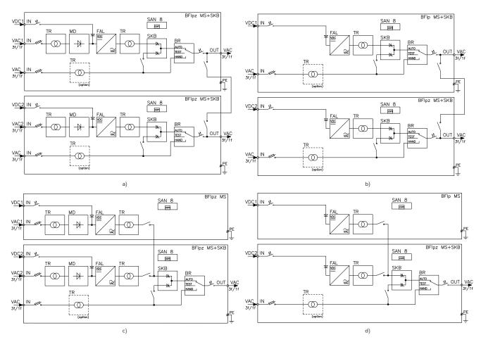
Fig. 67. Block diagram of the BFlpz / BFlp type inverter cabinets in a free design for parallel operation with the SKB type bypass. Possible configurations: a) a parallel system of two BFlpz inverters with own bypasses; b) a parallel system of two BFlp inverters with own bypasses; c) a parallel system of two BFlpz inverters with a single common bypass; d) a parallel system of two BFlp inverters with a single common bypass.
