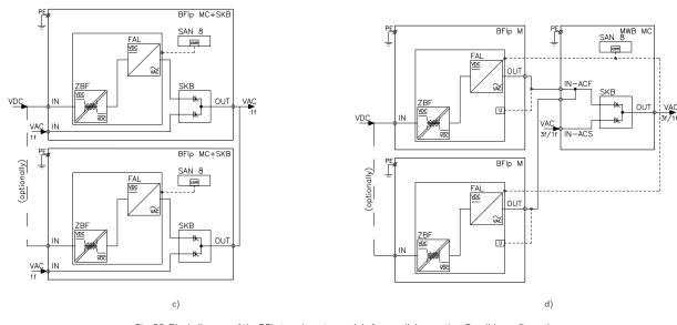
Fig. 50. Block diagram of the BFlp type inverter module for parallel operation. Possible configurations: a) two autonomous SKB type bypasses, a console built in the inverter module; b) a common SKB type bypass, a console built in the MWB module.
