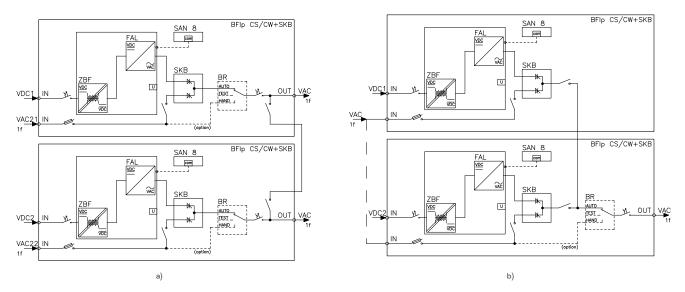
Fig. 75. Block diagram of the BFIp type inverter compact for parallel operation with the SKB type bypass. Possible configurations: a) two autonomous maintenance bypass switches, a built-in console; b) a common maintenance bypass switch, a built-in console.
