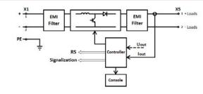
Fig. 24. Conceptual diagram of the converter without the EPIs type galvanic insulation
