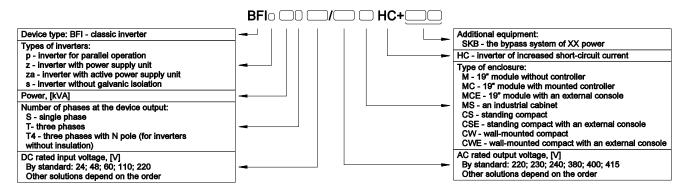
The HC version BFIz / BFI inverter modules create a family of devices, which, contrary to standard inverter modules, are characterised by increased operating parameters:
