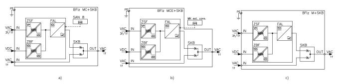
Fig. 46 Block diagram of the BFIz type inverter module with a power supply unit and the SKB type bypass: a) with a built-in console; b) with an external MK console; c) without a console.
