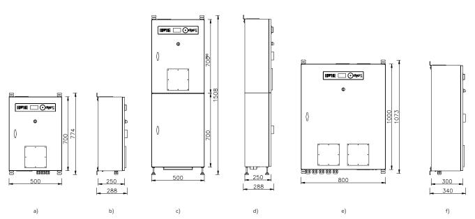
Fig. 76. Views with dimensions of the BFlpz / BFlp type inverter compact: a) CW6 compact – front view; b) CW6 compact – left-side view; c) CS6 compact – front view; d) CS6 compact – left-side view; e) CW1 compact – front view; f) CW1 compact – left-side view.
