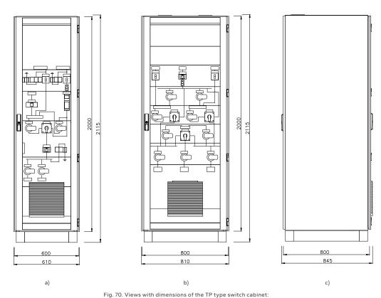
a) 600×800×2,000 cabinet – front view; b) 800×800×2,000 cabinet – front view; c) cabinet of depth of 800 mm – left-side view.
