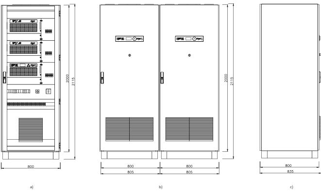
Fig. 69. Views with dimensions of the BFlpz / BFlp type inverter cabinet: a) 800×800×2,000 cabinet (modular design) – front view; b) (2×800)×800×2,000 cabinet (free design) – front view;
