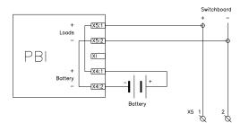
Fig. 3. A rectifier with an internal battery current measurement
