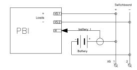
Fig. 4. A rectifier with an external battery current measurement
