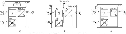
Fig. 101. Block diagram of the FAT type drive inverter module with a power supply unit: a) with a built-in console; b) with an external MK console; c) without a console.
