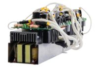
View of the PBI rectifier power block
