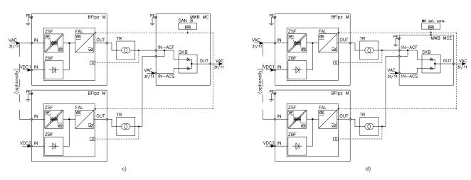
Fig. 55. Block diagram of the inverter modules for parallel operation with the BFlpz power supply unit and the MWB module. Possible configurations: a) power supply unit, battery converter, built-in console; b) power supply unit, battery converter, external MK console; c) power supply unit, diode in the DC power supply circuit, built-in console; d) power supply unit, diode in the DC power supply circuit, external MK console.
