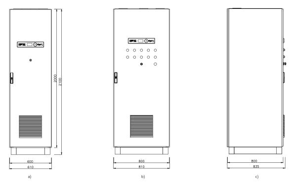
Fig. 97. Views with dimensions of the HPI type frequency converter cabinet: a) 600×800×2,000 cabinet – front view; b) 800×800×2,000 cabinet – front view; c) cabinet of depth of 800 mm – left-side view.
